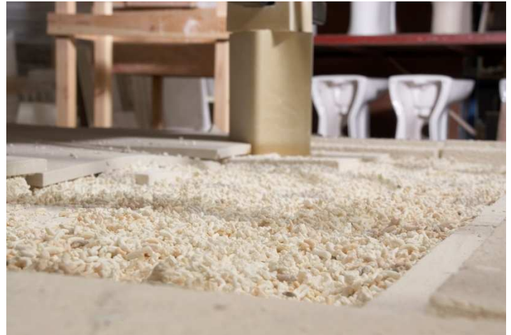
Photo showing the Kiln Car base now filled with Ultralite™ ROK
