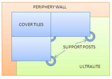
Plan View - Kiln Car Section showing typical position of Cover Tiles and Support Posts
